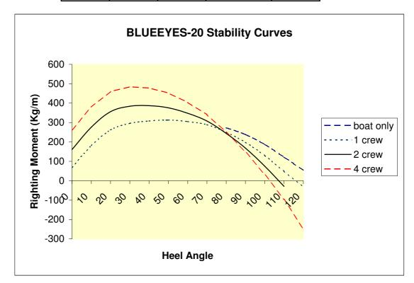
Notes: Sea condition will significantly impact possibility of capsize. Centreboard assumed to be locked fully down at all angles of heel.
